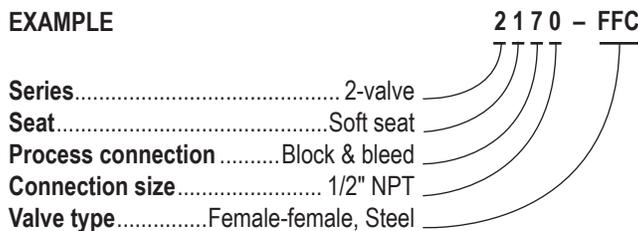
To meet all of your specific application requirements, the following **additional options** are available for these needle valves. To order all or any of these options, simply add them to the part number as shown in the diagram below.
