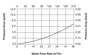
Curves represent nominal values, generated using water at 20°C. Characteristics may change under different operating conditions.
