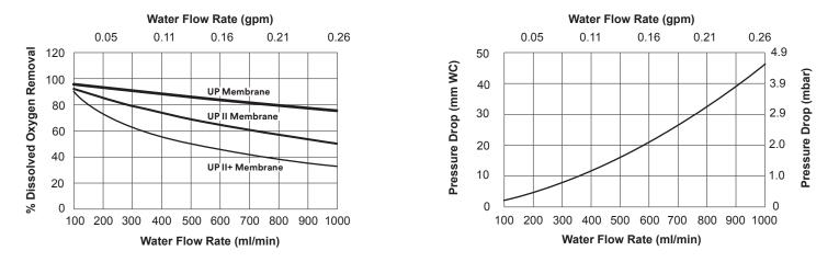
Test condition O<sub>2</sub> Removal: Vacuum mode with water at 45°C. Vacuum: 50 torr
