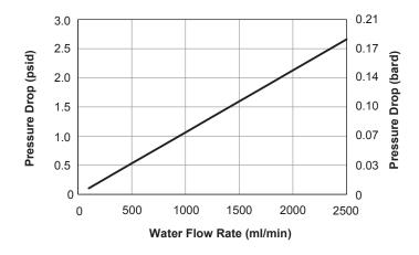
Curves represent nominal values, generated using water on the Lumenside at 20°C with 50 torr of vacuum drawn on both Shellside ports. We have plotted an estimated vacuum volume guideline that is based on a flow rate at 20°C, 50 Torr. Characteristics may change under different operating conditions.
