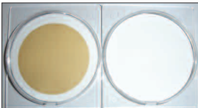
Varnish contained in fluid samples before and after treatment with Pall VRF system
