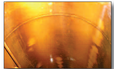
Filter housing internals coated with varnish
