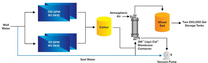
Additionally, the system was designed to operate with vacuum assisted air sweep, using a liquid ring vacuum pump to draw atmospheric air through the 3M™ Liqui-Cel™ Membrane Contactors.
